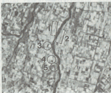
Photo 5 Landsat MSS band-5 & -7 imagery of site Y in Photo 1 - Sites 1 through 5 are flooded area reconized.
