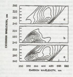
Fig.1. TLS-signatures of natural waters from different aquatoria (remote mode) and of oil dissolved in bi-distilled water (laboratory catalog): a) pure aquatorium near Lahemaa National Park (Estonia);
